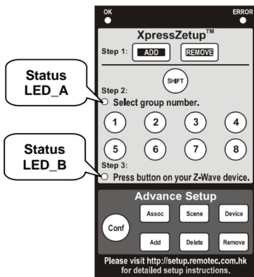
Figure 2 Setup Keys of the Z-URC™ 550EU
