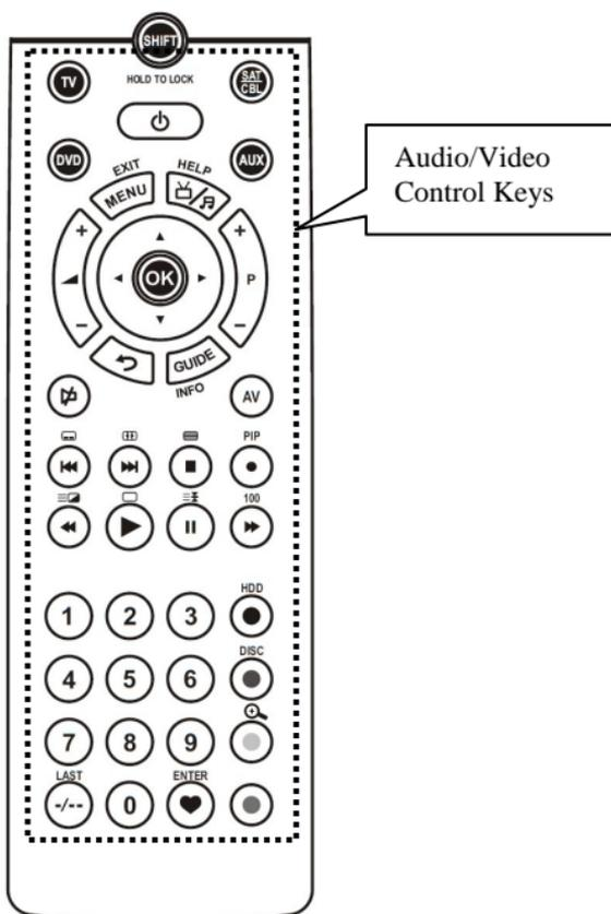
Figure 5 Audio/Video Control Keys of the Z-URC™ 550EU
