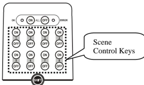
Figure 4 Scene Control Keys of the Z-URC™ 550EU
