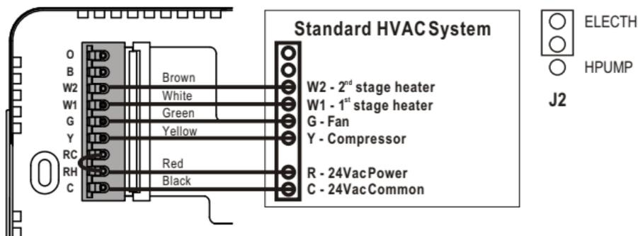
Figure 5. Heat pump HVAC system wiring
